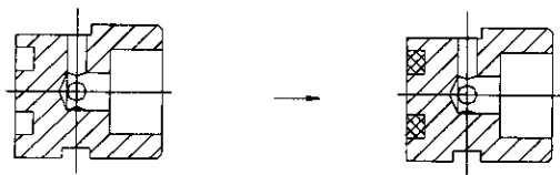
图2 工艺方案更改后阀芯结构 Fig.2 Current structure of valve core
