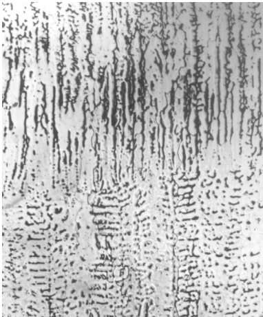
图 4 盖面层焊缝区组织 Fig.4 Welds zone tissue of capping beds
