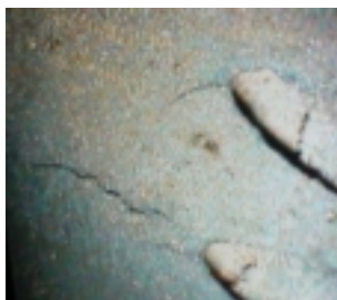
图 1 某产品内腔表面裂纹 Fig.1 Surface crack of cavity
