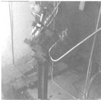
图 5 层板催化剂床热试车 Fig.5 The hot-firing of platelet catalyst bed
