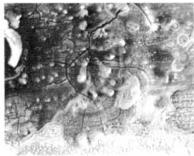
图 7 四氯化碳模拟件锈蚀产物形貌 Fig.7 Rusting appearance of carbon tetrachloride analog specimen
