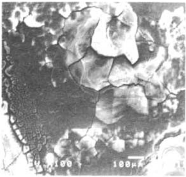
图 1 锈蚀件表面锈斑形貌 Fig.1 Rusty spot on rusting part surface
