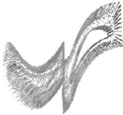
图 7 静子与转子间相对速度的分布 Fig.7 Relative velocity distributions between a stator and a rotor
