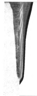
图 6 模拟的熔池形貌与实际焊缝金相形貌对比图片 Fig. 6 Comparison of simulated weld shape with actual weld joint metallographical morphology
