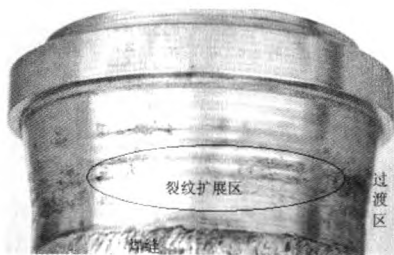
图 1 阀门肩圈连接端出现的裂纹 Fig. 1 Flaw at valve shoulder ring connection end
