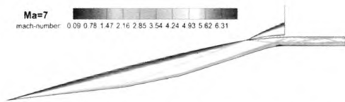
图 4 Ma=7.0 时平移唇口进气道的流场 Fig. 4 Flow field of the inlet with translating cowl at Ma=7.0
