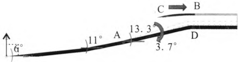
图 8 2.5\leq Ma\leq 4.0 时变几何进气道的构型 Fig. 8 Configuration of variable geometry inlet with at Mach number 2.5~4.0
