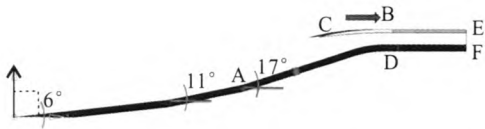
图 10 6.0\leq Ma\leq 7.0 时变几何进气道的构型 Fig. 10 Configuration of variable geometry inlet at Mach number 6.0~7.0
