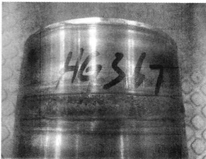
图 5 HGH367 焊丝所焊试验件的焊缝表面 Fig. 5 Specimen weld joint surface made through with HGH367 welding wire
