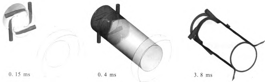
图 2 敞口型离心式喷嘴液体填充过程 Fig. 2 Process of liquid phase filling into open type pressure swirl injector
