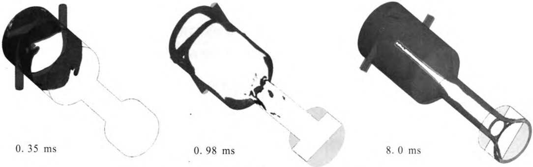
图 5 收口型离心式喷嘴液体填充过程 Fig. 5 Process of liquid phase filling into closing-in type pressure swirl injector
