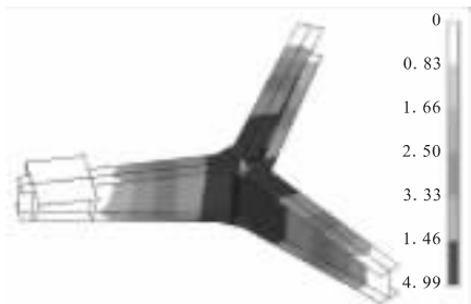
图 4 复合材料机架在飞行工况载荷下变形图 Fig. 4 Deformed shape of composite thrust frame under flight conditions
