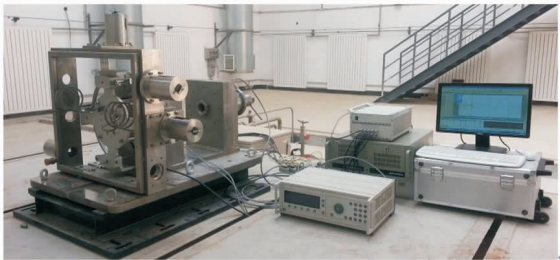
图4 矢量推力测量与校准系统 Fig.4 Vector thrust measurement and calibration system
