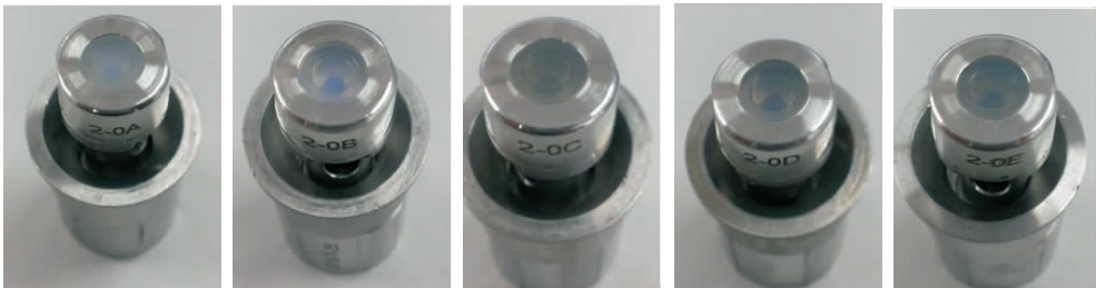
图 2 五种原料加工成的阀芯组件 Fig. 2 Valve core components made from five materials
