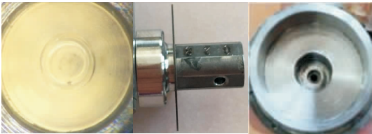
图 4 试验后阀门分解情况 Fig. 4 Disassembled valve after life test
