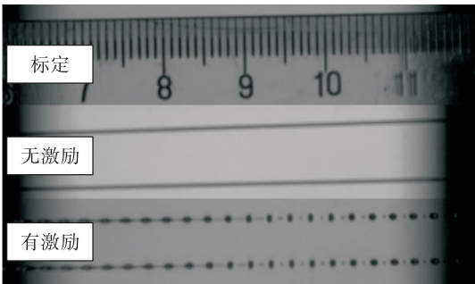
图 4 压电激励对真空射流状态的影响 Fig. 4 The influence of piezoelectric excitation on the vacuum jet shape
