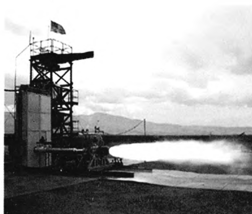
图 4 NOFBX 大推力发动机热试车台 Fig. 4 Hot test equipment of large thrust NOFBX engine
