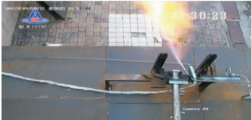
图 6 通入液氧后的火焰形态 Fig. 6 The picture of gas after the inflow of liquid oxygen
