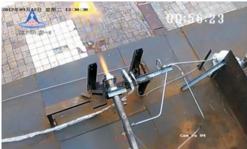
图 15 液氧与燃气补燃瞬间 Fig. 15 The time of spontaneous combustion of liquid oxygen and gas
