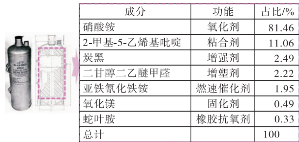
图 3 M15A1-JATO 结构及推进剂成分 Fig.3 Structure and propellant composition of M15A1-JATO
