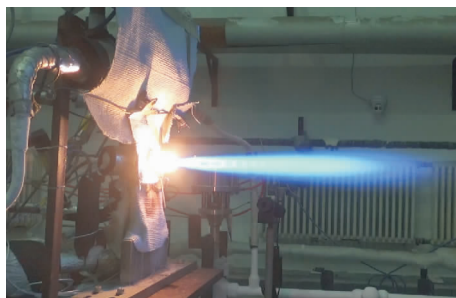
图12 150 N 发动机(铌钨合金燃烧室)稳态热试车 Fig.12 Steady-state hot-fire test of 150 N LOx/LCH 4 engine with niobium-tungsten alloy combustion chamber
