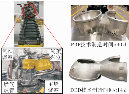
图 3 PBF 技术和 DED 技术制造 RS25 发动机推力室头部比较 Fig. 3 Comparison of the thrust chamber head in RS25 engine manufactured by PBF technology and DED technology
