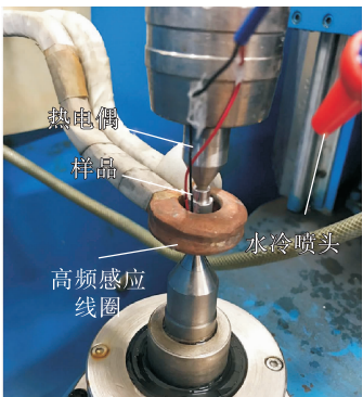
图 1 激光定向能量沉积设备、Stellite 6 粉末及热疲劳试样 Fig. 1 Laser directed energy deposition equipment, Stellite 6 powder and thermal fatigue sample
